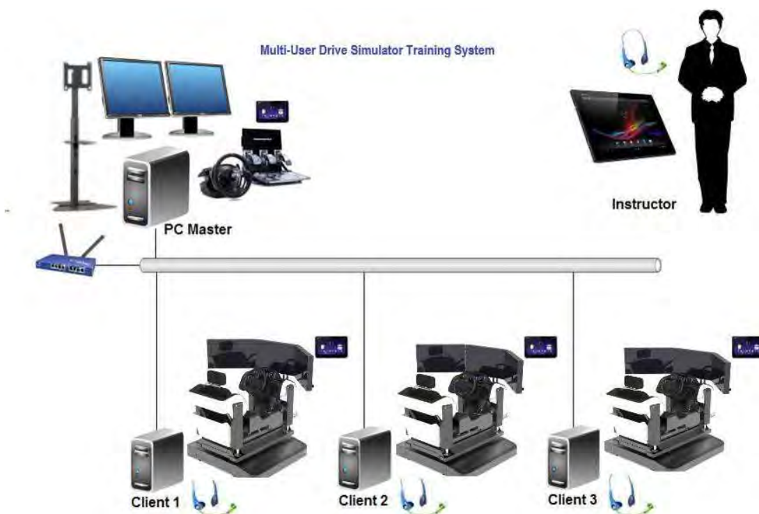
A typical Multi-Driving Simulation & Instructor Control System
