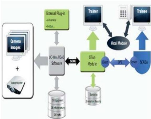
**Figure 6:** G'Val Standard Software Architecture
