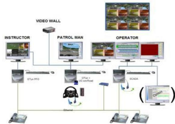
Figure 5: G'Val Standard Hardware Architecture
