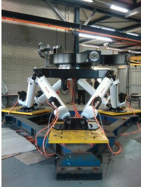
The 6 DOF hexapod undergoing final factory testing at Bosch Rexroth
