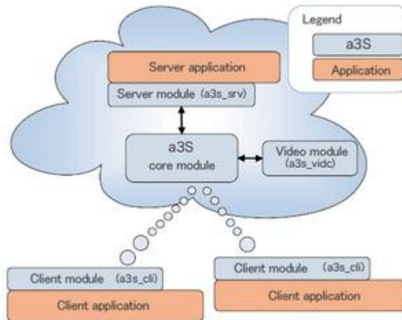
Figure 6 System configuration
