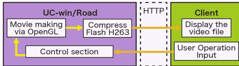
Figure 2 Mechanism of data transmission during driving simulation on cloud (Conventional type)
